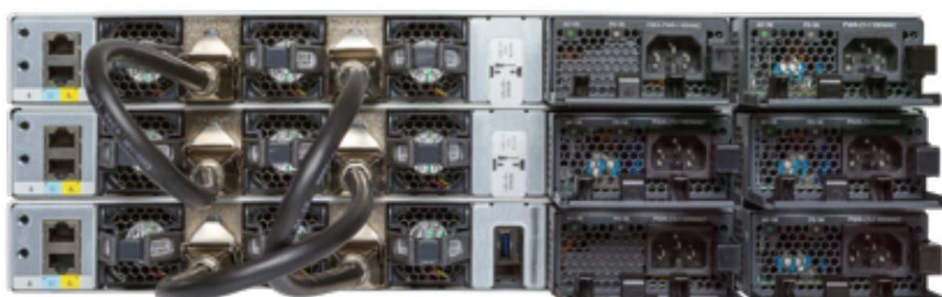
Figure 5. Cisco Catalyst 9300 Series switch stack units
