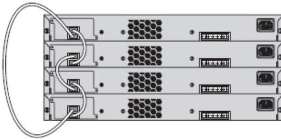
The 0.5-meter cable can be used to connect two Cisco Catalyst 2960 switches that are 4 rack units away from each other. In a stack of four, with all four members racked directly on top of each other, 0.5-meter cables can be used to connect all stack members. When stack members are more than 4 rack units apart, then longer stack cables are required.
