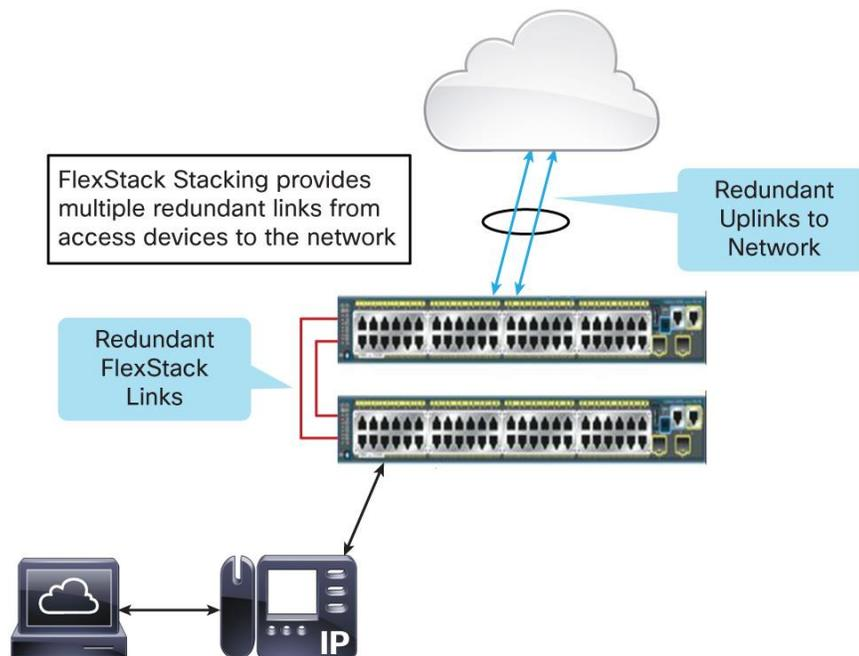
Flexibility of FlexStack allows for modular stacking capability. Cisco Catalyst 2960 switches can be added to a stack at any time by adding the optional FlexStack module. As the demand for Ethernet access ports increases, Cisco Catalyst 2960 switches can be stacked together either to create a new stack or to add new Cisco Catalyst 2960 switches to an existing stack. This flexibility provides investment protection for the network administrator, who can add additional stack members as needed.
