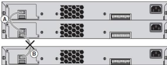
Since the stack in the connection in Figure 12 has broken into two, only two members will have their stack port status shown. The third member has been removed from the stack.
