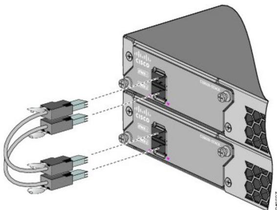
When each member in the stack has two operational FlexStack links, then the stack is operating in a fully redundant mode. The dual FlexStack connections from each member to two other members are what provide the redundancy. Should any single FlexStack connection break or cease to operate, then the switches in the stack will use the remaining FlexStack connection that is provided.
