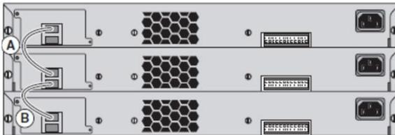
Three different FlexStack-Plus cable lengths are available, as shown in Table 4.
